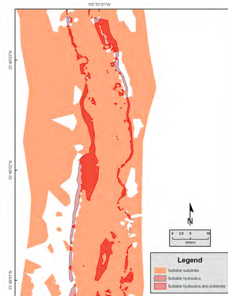
Figure 17. Example of an intersection map of areas having suitable hydraulic and substrate conditions for speckled dace ( Rhinichthys osculus ) in a portion of the upper (Gage) site at a discharge of 100 cubic feet per second.
